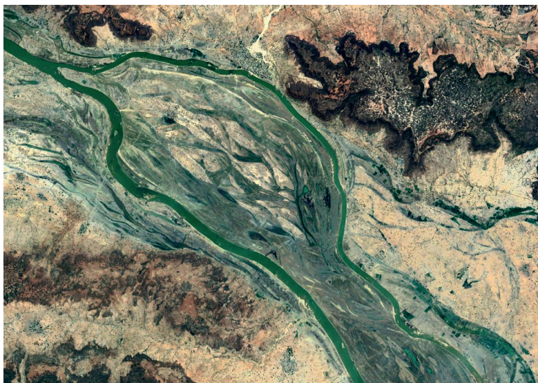
Figure 2.7 The multi-thread braided channel of the Niger river where it marks the boundary between Benin and Niger near Ouna, Niger. Image: Google, CNES/Airbus.
